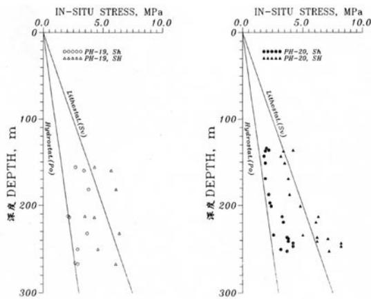
Figure4 Correlation between in-situ Stress Magnitude and Depth
