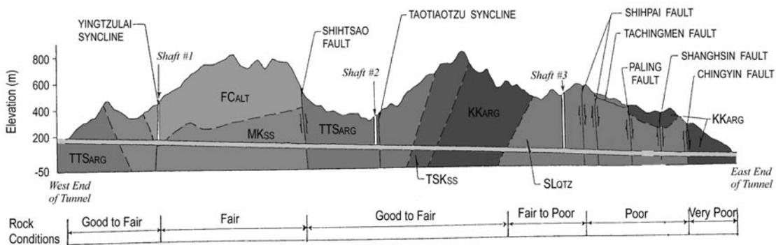
Figure 7 Geological Profile along the Hsuehshan Tunnel
