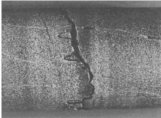
Figure 3 Stylolite in the Vertical Drill Core of Szeleng Sandatone
