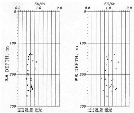
Figure 5 Correlation between Stress Ratio and Depth
